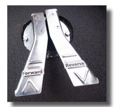
**TRAVEL CONTROL**Dual hydraulic transmission foot controls are more responsive and comfortable for operator comfort.
