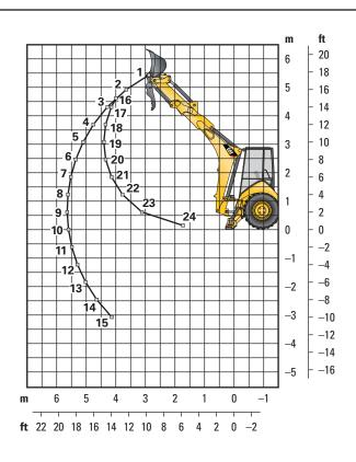
Lift Capacities are over-end values. Machine equipped with 4WD, OROPS, 0.96 m<sup>3</sup> (1.25 yd<sup>3</sup>) general purpose bucket, and no counterweight. Extendible stick includes 460 kg (1,015 lb) counterweight.
