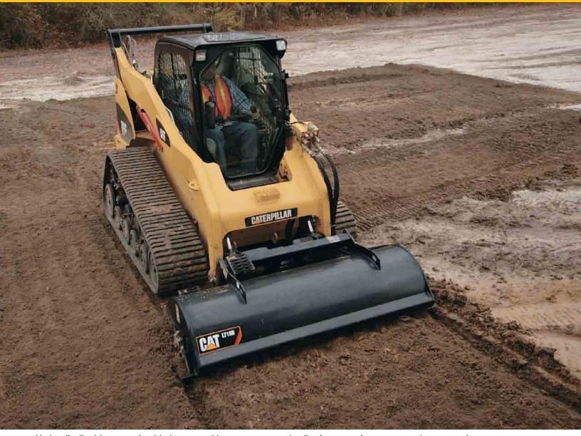
Hydraulically driven rotating blades cut and loosen compacted soil prior to sowing grass or other vegetation.
