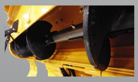
Optional remix chamber provides a consistent mix of material to the paver. Chamber hydraulically moves into position and includes an increase to 137 HP (102 kW)
