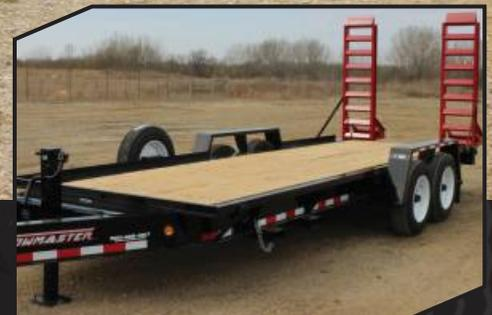
84" load width option on T-14D and T-16D includes an open-fender design.
