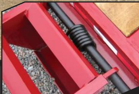
Spring-assist heavy-duty ramps are standard.
