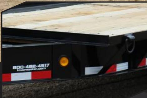
Cold-formed one-piece I-beam tongue and main frame provide the strength you need to haul your equipment.
